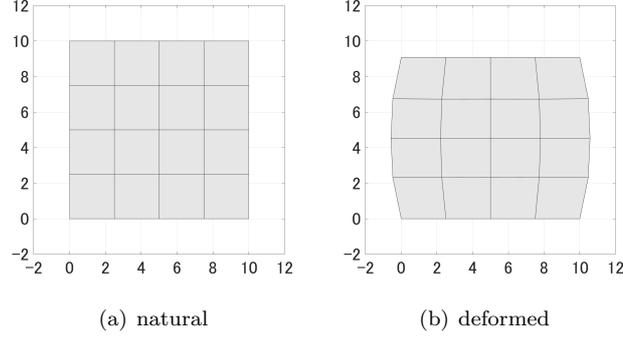
Figure 3.14: Deformation in push test under rectangle elements
