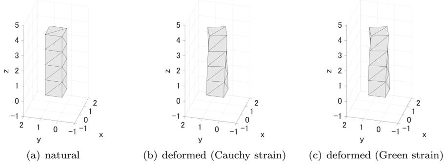
Figure 3.19: Twisted beam
