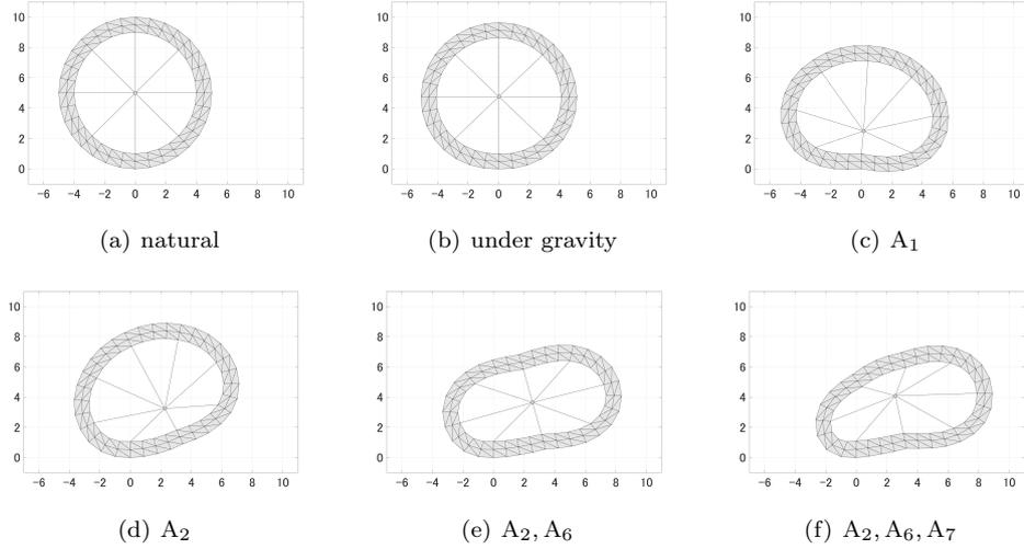
Figure 3.11: Elastic ring deformed by spring actuators
