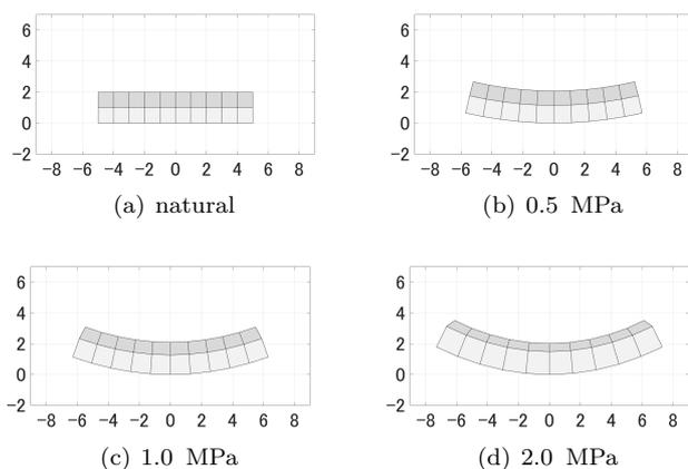
Figure 3.16: Deformation by inner pressure of layered body
