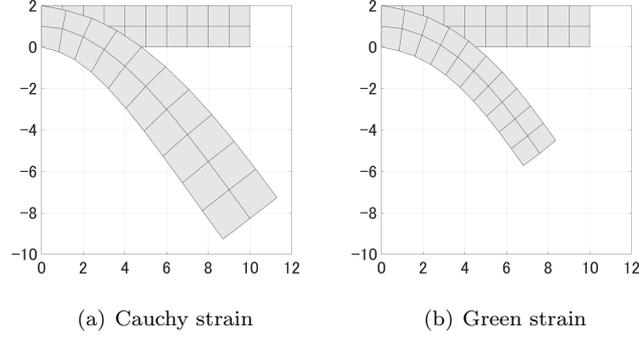
Figure 3.15: Calculation via Cauchy and Green strains using rectangular elements
