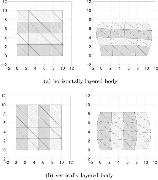
Figure 3.8: Deformation of layered bodies in push test
