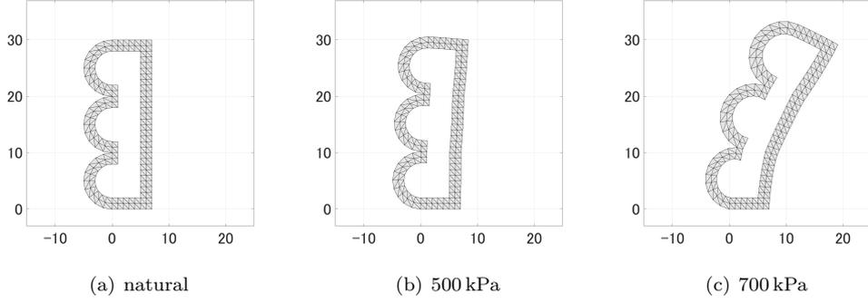
Figure 3.7: Deformation of PneuNet actuator
