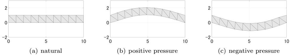
Figure 3.6: Deformation of membrane by pressure
