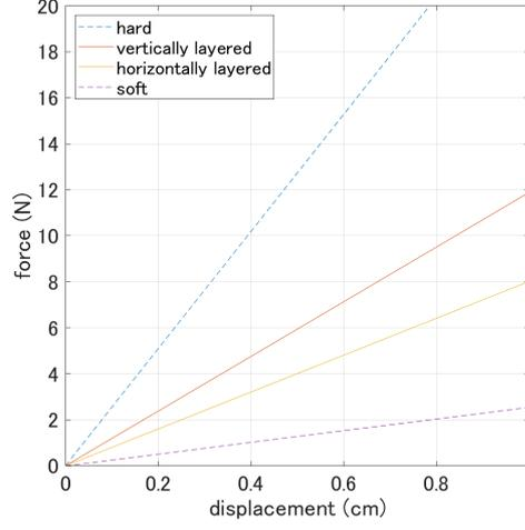
Figure 3.9: Force-displacement relationship in push test
