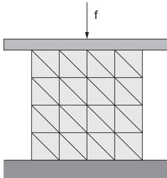
Figure 3.3: Push test of an elastic body
