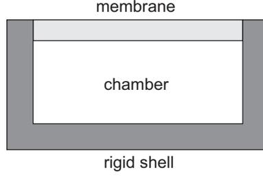
Figure 3.5: Elastic membrane deformed by air pressure
