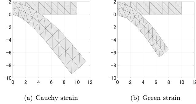
Figure 3.10: Computation via Cauchy and Green strains
