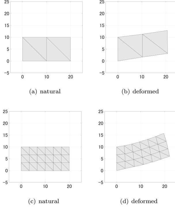
Figure 3.1: Calculated deformation of a rectangular elastic body
