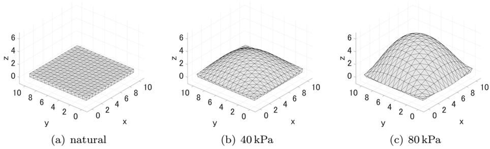
Figure 3.20: Expansion of an elastic membrane under pressure
