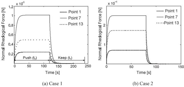
**Fig. 6** Normal rheological forces on the bottom surface in both simulations. Rheological force increases quickly in push phase and converges to a constant value. In keep phase, rheological force decreases quickly to zero.
