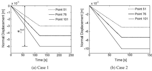
**Fig. 5** Normal displacements of some nodal points in both simulations. In push phase, displacements of all points increase with a constant velocity. In keep phase, displacements keep constant and there is no displacements recovery after releasing.
