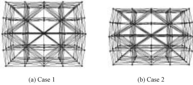
**Fig. 4** Deformed shapes in both simulations. (a) Final deformation with parameters:  $E = 8 \text{ Pa}$ ,  $c_1 = 5 \text{ Pa}\cdot\text{s}$ ,  $c_2 = 40 \text{ Pa}\cdot\text{s}$ , and  $\gamma = 0.43$ . (b) Final deformation with parameters:  $E = 300 \text{ Pa}$ ,  $c_1 = 200 \text{ Pa}\cdot\text{s}$ ,  $c_2 = 500 \text{ Pa}\cdot\text{s}$ , and  $\gamma = 0.35$ .
