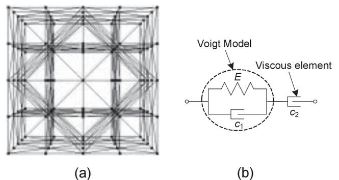
Fig. 3 3D FE mesh and three element model. (a) FE mesh includes 125 mass points, 64 parallelepipeds and 384 tetrahedrons. (b) Three-element model which can be employed to describe linear rheological deformation.
