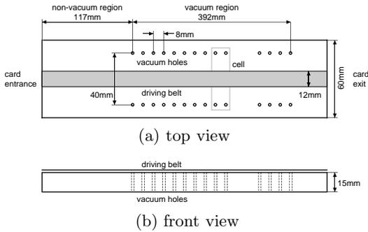
Figure 4: Arrangement of vacuum holes
