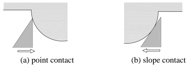
(a) point contact (b) slope contact Fig. 6 Two types of contact between a micropart and a sawtooth
