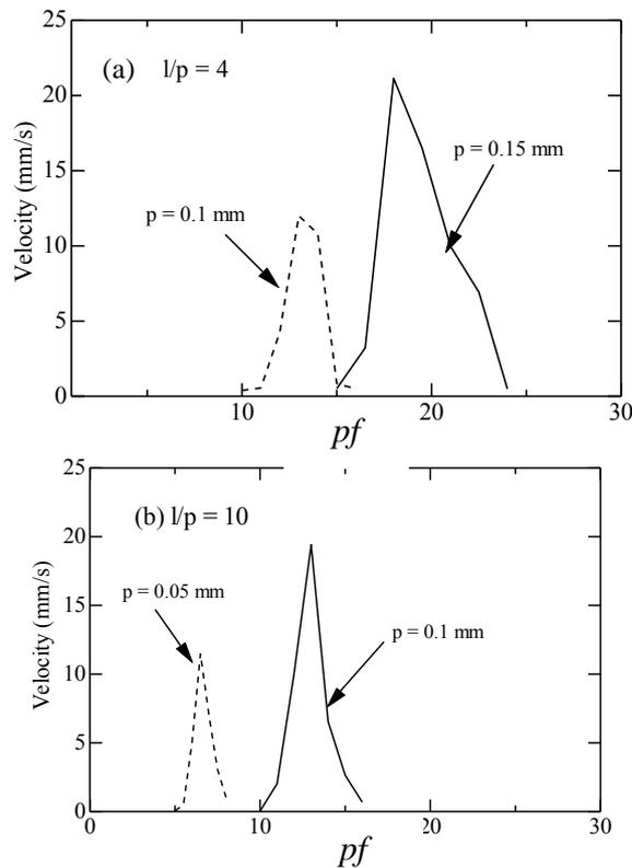
Fig. 4 The analysis feeding micro-parts for the same value of ratio  $l/p$  runs with frequencies: (a)  $l/p = 4$ , (b)  $l/p = 10$ .
