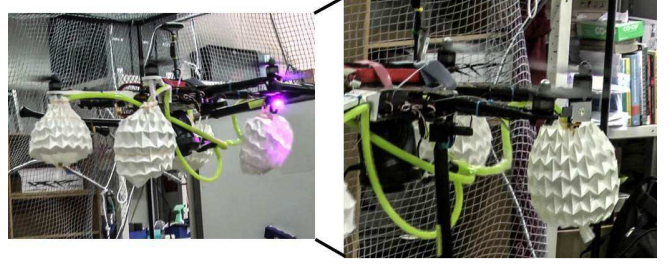
Fig. 8 Deflated Origami ball while the helicopter takes off and flies
