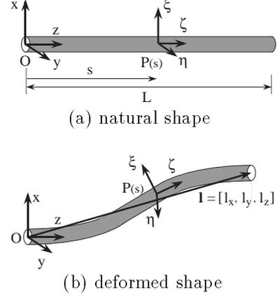
Figure 1: Description of relationship between natural shape and deformed shape
