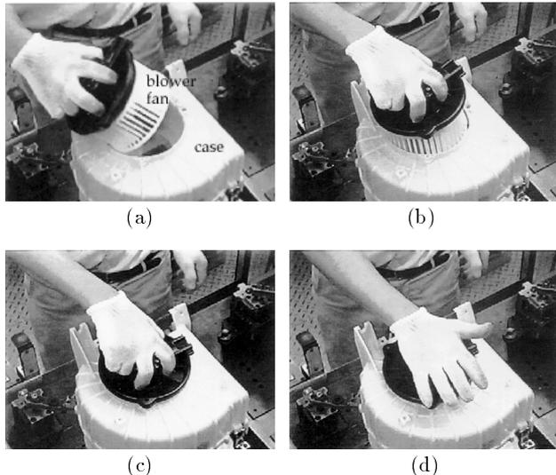
Figure 3: Insertion of blower fan into case
