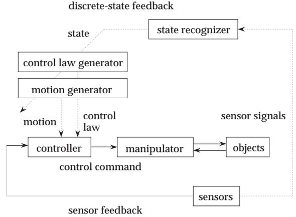
Figure 2: Sensor feedback and discrete-state feedback
