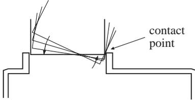
Figure 6: Motion of blower fan in human insertion
