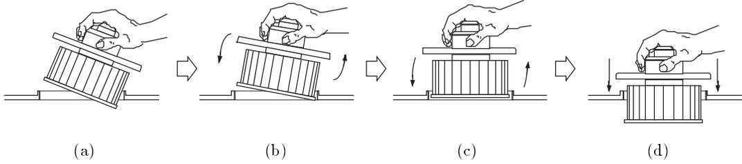
Figure 5: Process of human insertion of blower fan
