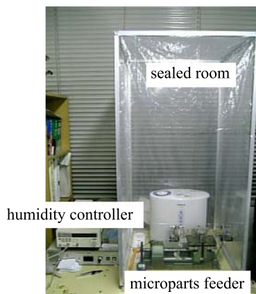
Fig. 2 Humidity control system
