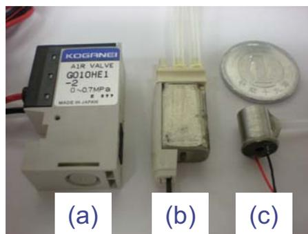
**Fig.1** Comparison of pneumatic valves: (a) solenoid valve (dimensions  $32 \times 26 \times 10$  mm), (b) pilot-operated solenoid 3/2 DCV (dimensions  $32 \times 12 \times 7$  mm), and (c) prototype miniaturized unconstrained valve (dimensions  $\phi 7 \times 9$  mm)
