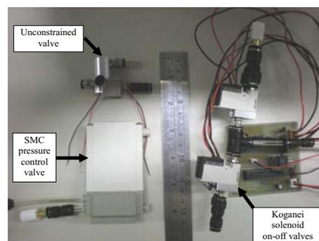
**Fig.6** Unconstrained valves having the smallest size among the pressure control devices
