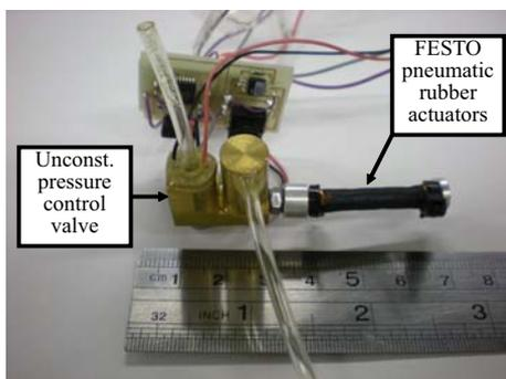
Fig.7 Miniaturized pneumatic servodrive
