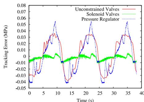
**Fig.5** Comparison of pressure tracking error at 50 mHz
