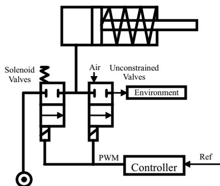
Fig.2 Unconstrained valves for control of a single-acting pneumatic cylinder
