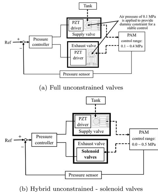
Fig.3 Implementation combinations of unconstrained valves for pressure control valves
