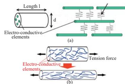
Fig.1 Model of a a tension-sensitive electro-conductive yarn.
