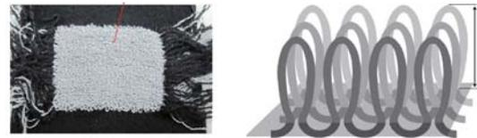
Fig.4 Slip sensor with piles shaping the surface.
