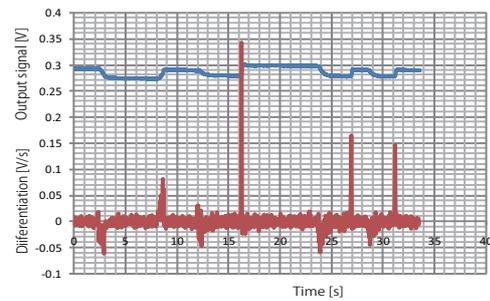
Fig.7 Output of the sensor and its differentiation during load/unload action.
