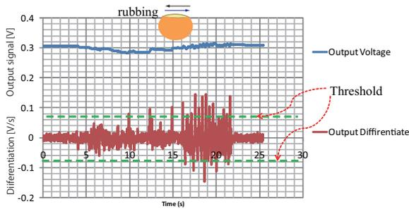
Fig.6 Output of the sensor and its differentiation during rubbing action.
