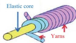
Fig.3 Yarn with double coupling structure.
