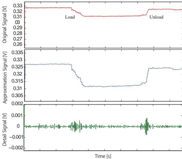
Fig.8 Output of the sensor and DWT signals during load/unload test.
