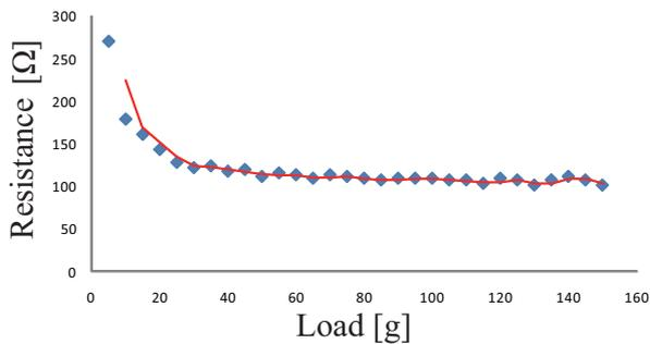
Fig.2 Relation of resistance and load in the tensile experiment, and its fitting curve.
