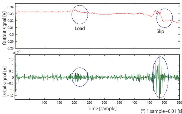
Fig.9 DWT signal of one loading and sliding test.
