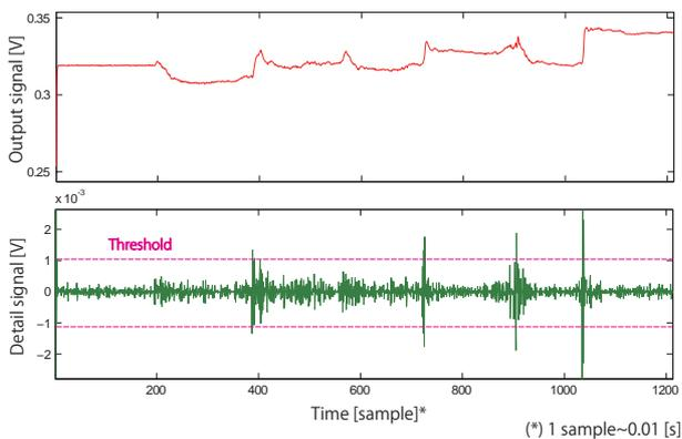
Fig.10 DWT signal during rubbing action.
