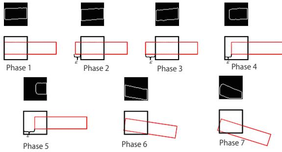
Fig. 7. Postures of the grasped object through phases.
