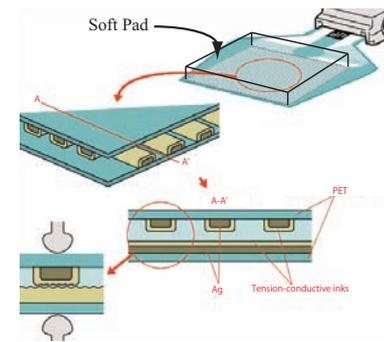
Fig. 1. Nitta<sup>®</sup> tactile sensor with the soft pad. This image was edited from the original one in [5]
