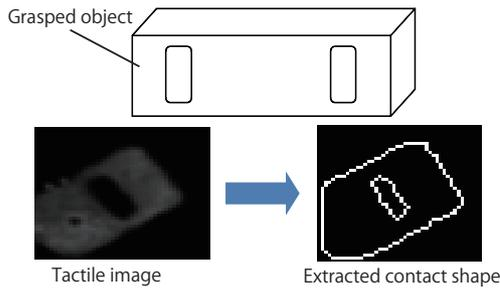
Fig. 4. Contact shape detection in term of boundaries.
