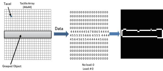
Fig. 2. The similarity between a tactile data and a grayscale image.
