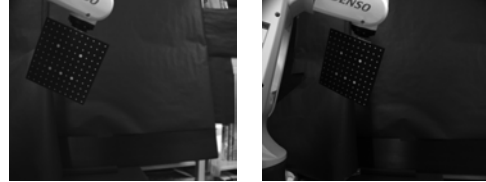
(a) Left image (b) Right image Fig. 4 Stereo images to use for camera calibration
