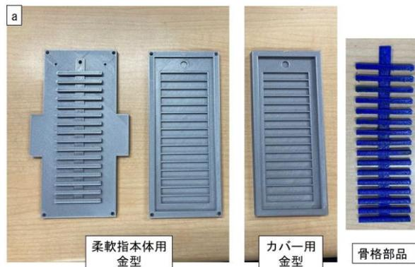
Fig.4 New method mold(a) and State of modeling of new method(b)
