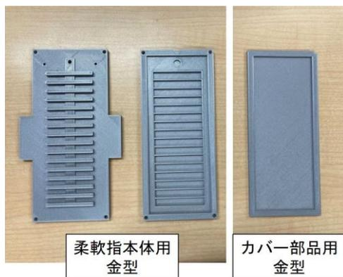
Fig.2 Conventional mold
