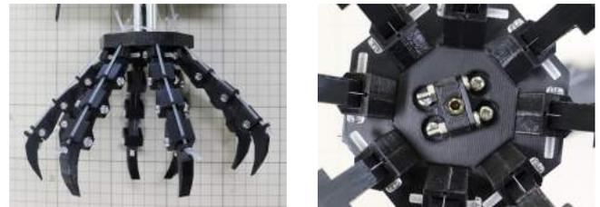
Fig.1: Proposed robotic gripper at its (a) front view and (b) bottom view showing the camera embedded in the center.
