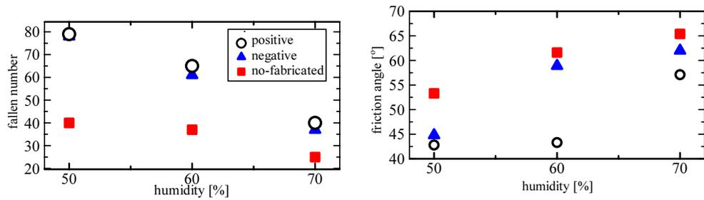
(a) Number of capacitors that fell from the microfabricated surface, of a total of 105 capacitors
