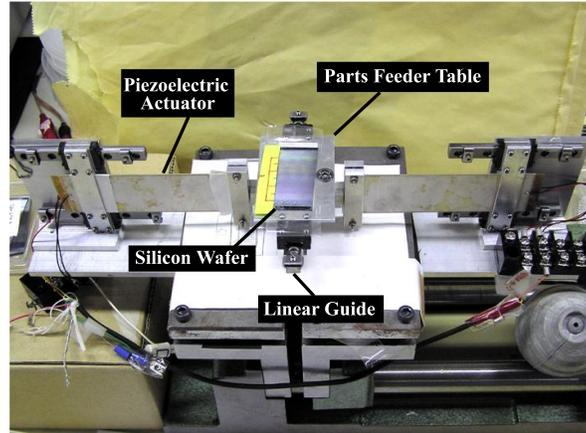
Figure 12. Micropart feeder using bimorph piezoelectric actuators
