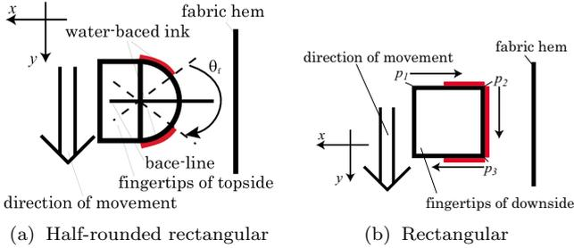
Fig. 5: Robot fingertips contact with hem of fabric
