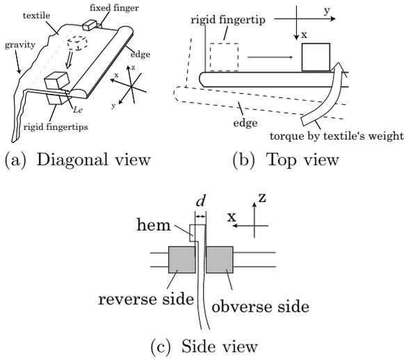
Fig. 1: Horizontal pinching slip motion for fabric unfolding
