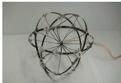
Fig.17: Spherical prototype for crawling and jumping
