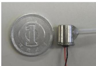
Fig.6 New miniaturized valve (φ7×9mm)
