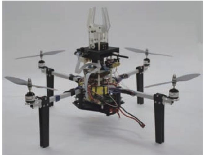
**Fig.1** Picture of the aerial robot with upward directed hand and camera.
