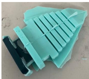
Fig.10 hand made by core insert mold
