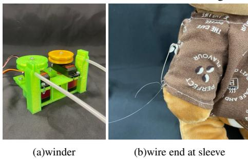
Fig. 8 Winding mechanism
