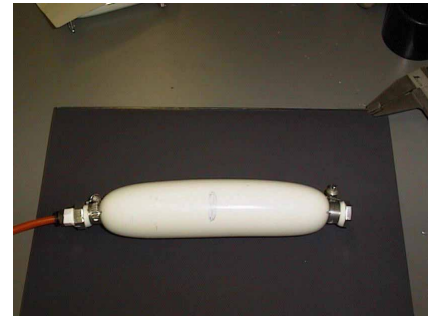
Fig.6 Deformed shape of sample 1 (Pressure 0.01[\text{kgf}/\text{mm}^2] )
