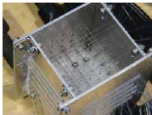
図 3.31: Mold and washer are used in making soft objects
