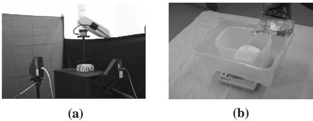
Fig. 7. (a) An experiment system: A real rheology object is pushed by a rectangular rigid body located at the tip of a robotic manipulator, and deformations of its sides are measured by two *Digiclops* cameras. (b) The volume difference between an initial real rheology object and its pushed one is measured by the overflowed water.
