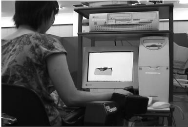
**Figure 11** : A human operator watches deformation of a rheology object by a 3-D graphics software *OpenGL* and feels its three forces and three moments by a six-degrees-of-freedom robotic arm *Joyarm*.
