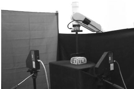
**Figure 5** : An experiment system: A real rheology object is pushed by a rectangular object located at the tip of a robotic manipulator, and side deformations are simultaneously measured by two *Digiclops* cameras.
