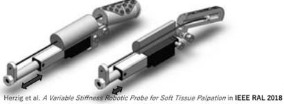
Herzig et al. A Variable Stiffness Robotic Probe for Soft Tissue Palpation in IEEE RAL 2018
